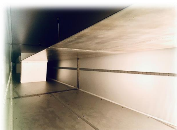
Figura 3. Interior Celda G-TEM
